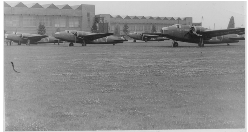
The Wellingtons pictured here are early models before the rotating gun turret replaced the single gun in the nose of the aircraft.
