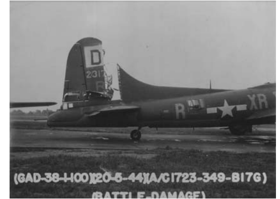
This is a good example of the type of damage inflicted in the B-17s
