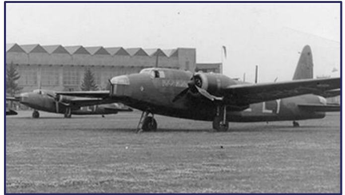
The Wellingtons pictured here are early models before the rotating gun turret replaced the single gun in the nose of the aircraft
